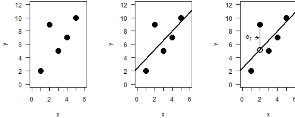
Figure 4.1: Left Panel: Plot of five points. Center Panel: Line of best fit through the data. Right Panel: Error of estimation for the second point.
